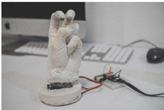
Fig 5. Hand sculpture that predicts where your interaction with it will stem from. Servo for rotation is controlled using a microcontroller that detects user distances using an ultrasonic sensor. The learning algorithm predicts future audience positions by keeping track of the averaged time series of previous responses. Sources: Ray LC.
