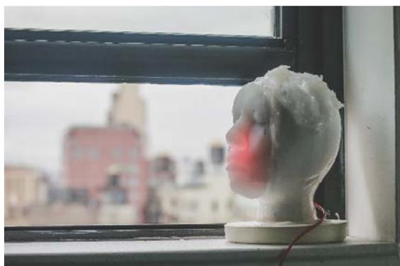
Fig 7. A head sculpture that uses computer vision to see where the audience is, and makes replies using digital code embodied as a LED matrix that sweeps across the mouth of the statue, representing machine communication.
