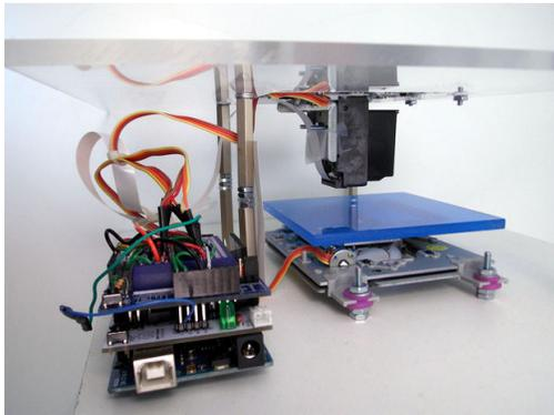
**Figure 1: A hypothetical bioprinter that accepts G Code commands line-by-line and extrudes edible material interactively, controlled via computer and Arduino.**
