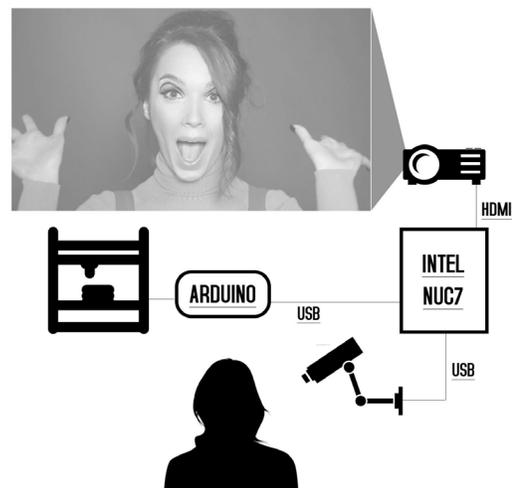
**Figure 2: Exhibit plan using a webcam to capture human face, detect emotions and expressions in Unity on the NUC7 computer, and use that to control motors in the bioprinter. Expressions can also be viewed for feedback on projection.**
